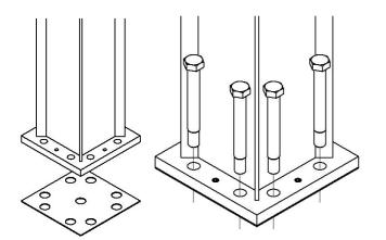
Alt 2. Direct Burial Mount - Do not use the Column Mount or Leveling Plate, continue to part 5. 3
